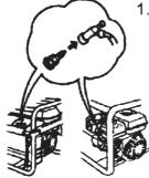
1. Remove the nut of spark plug.
